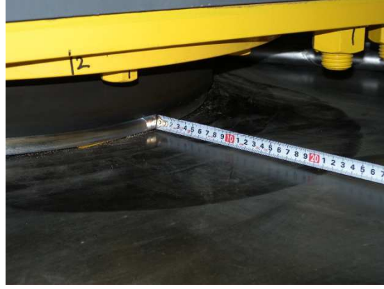
(b) Trace of movement of sliding damper
