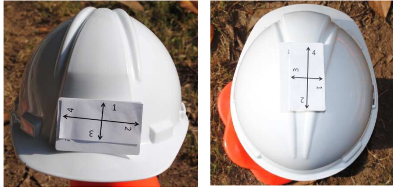
Figure 3: PPU mounted on a hard hat in the vertical position (left) and the horizontal position (right)
