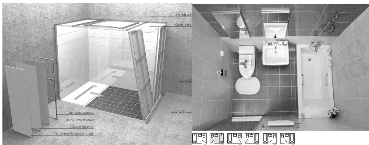
Figure 2: Potential modular bathroom system (Design type: Daelim Batos ® DBR)
