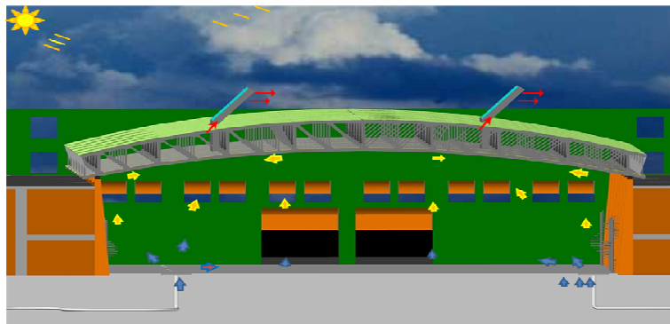
Picture 5: Exchangers-solar chimneys overall operating scheme
