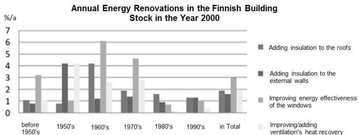
Figure 3. Annual energy refurbishments in the Finnish building stock in the year 2000. On average about 2% of measures are carried out annually. Windows are being improved more often than that. (Vainio et al. 2002)
