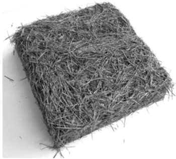
Figure 6. Prototype for mulched spinifex insulation batt. (Photo by Tim O'Rourke.)
