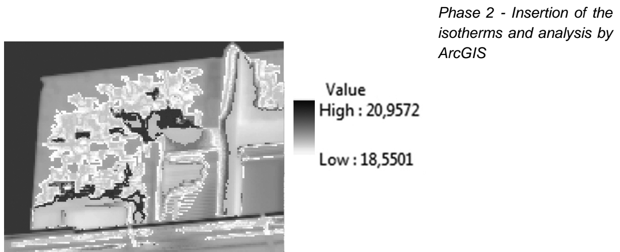
Figure 5: Building 14 North façade, 6 th floor – characteristic thermal gradient identification
